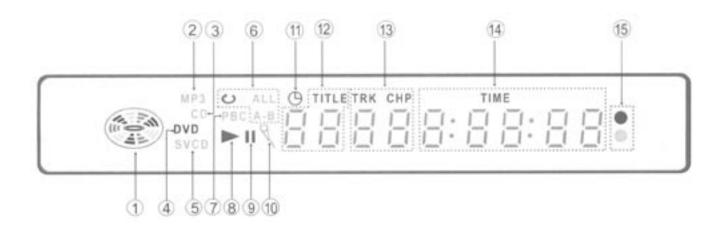
The figure above shows the front panel with all the displays on.
